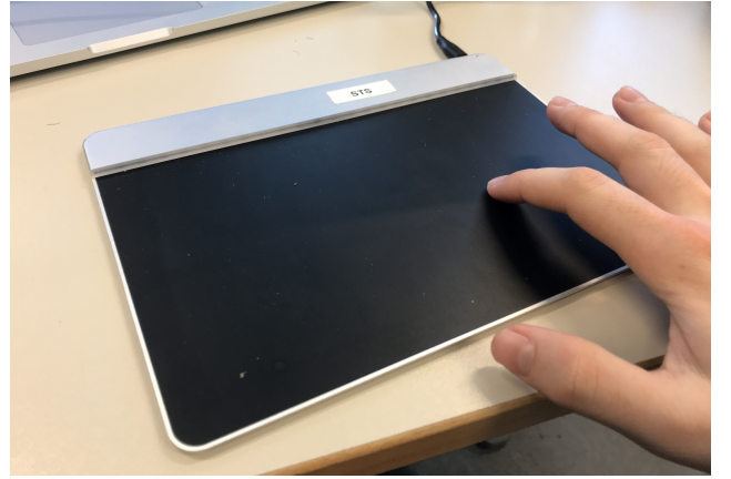
Figure 6: The Sensel Morph: an expressive touch sensitive controller used for controlling the real-time elasto-plastic bowed string implementation.
